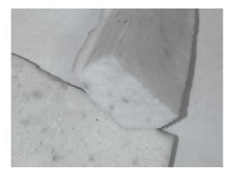
Fig. 5. Samples of heat insulating coatings on the basis of hollow glass microspheres with addition of foamed glass and liquid sodium glass as binder.
